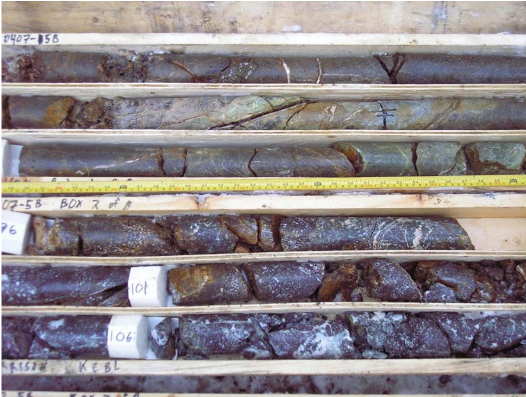
Photo I-14 Rock core from DH07-5B showing moderately weathered material
