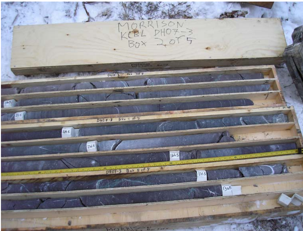
Photo I-11 Rock core from DH07-3A. Rock is purple with green staining
