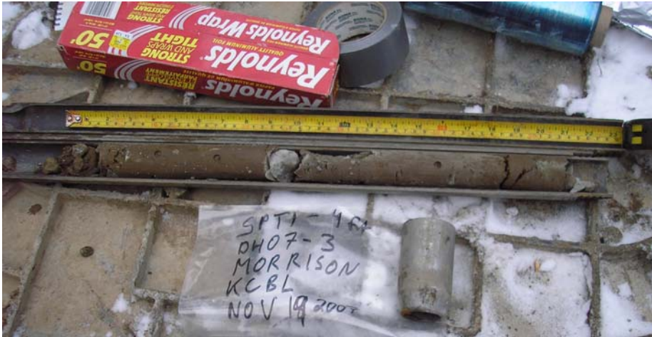
Photo I-8 SPT sample with broken gravel midway
