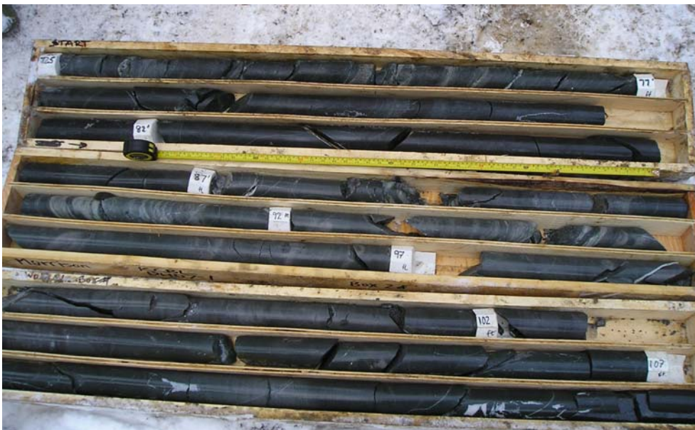
Photo I-9 Rock core from DH07-1A. Note the inclined stratification
