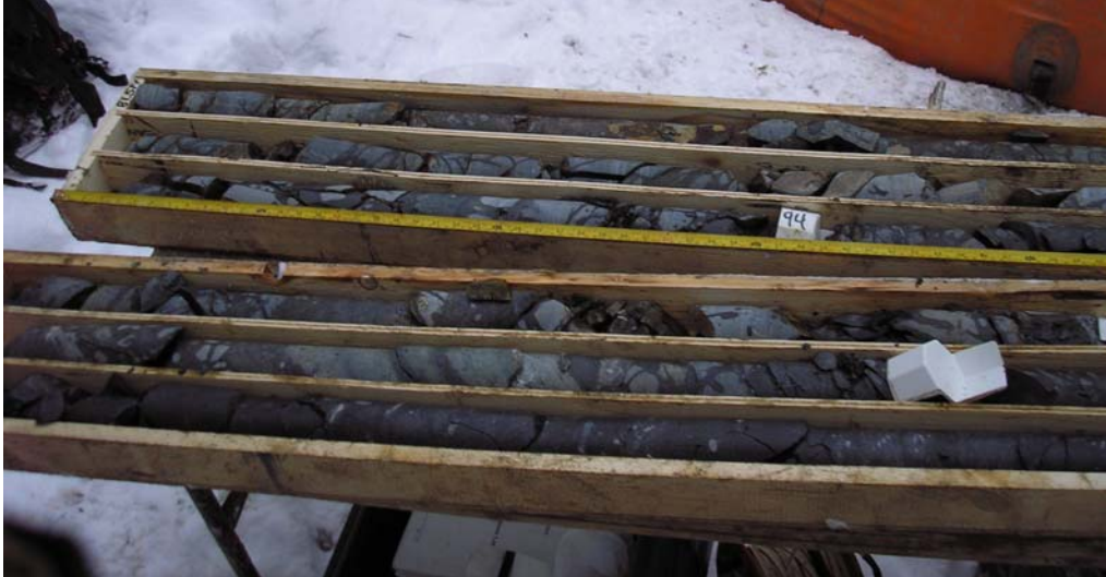
Photo I-10 Rock core from DH07-2. Rock is dark grey with joints filled with weathered calcite.
