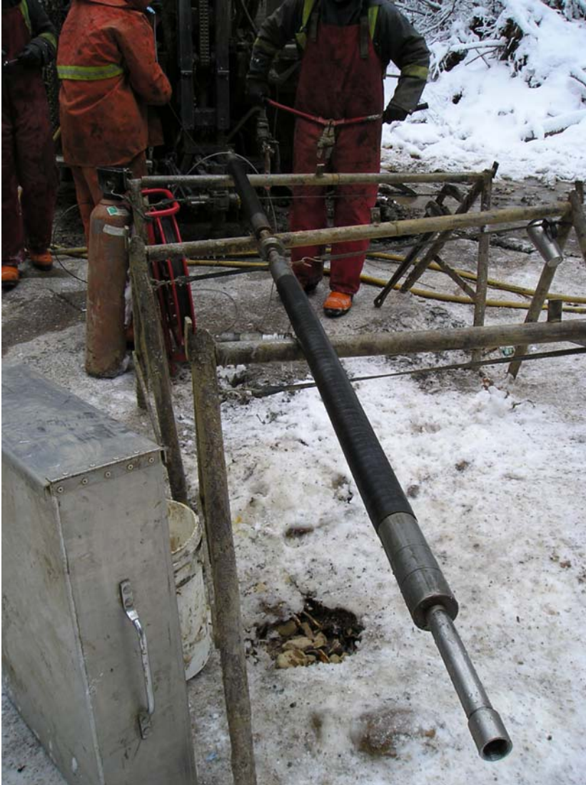
Photo I-18 Packer system. The metal ring between the two packers lands on the drill head. The upper packer inflates in the drill stem, and the lower packer inflates against the rock in the open hole.
