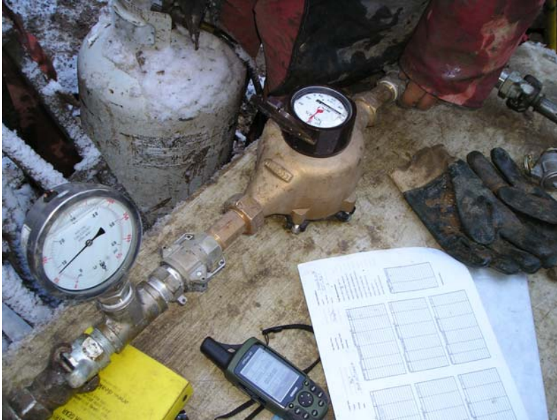
Photo I-20 The pressure and flow gauges used to perform the packer tests
