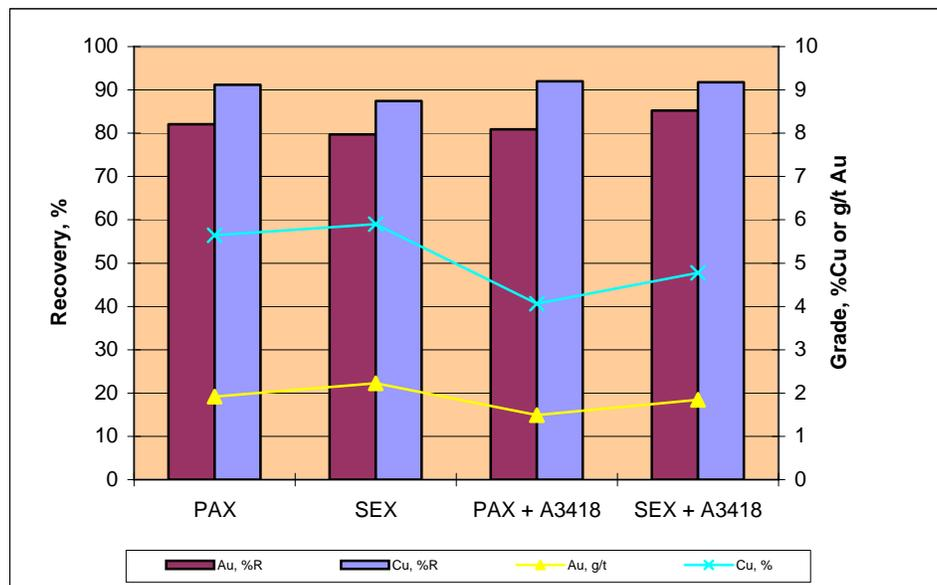
**Figure 4.7 Effect of Collector Types on MHM1C**
