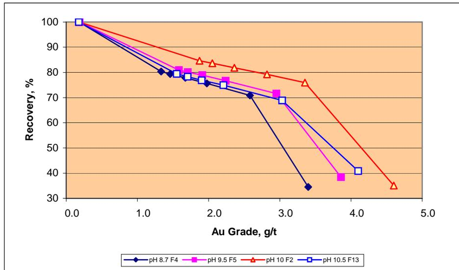
**Figure 4.5 Effect of pH on Au Flotation for MHM1C**
