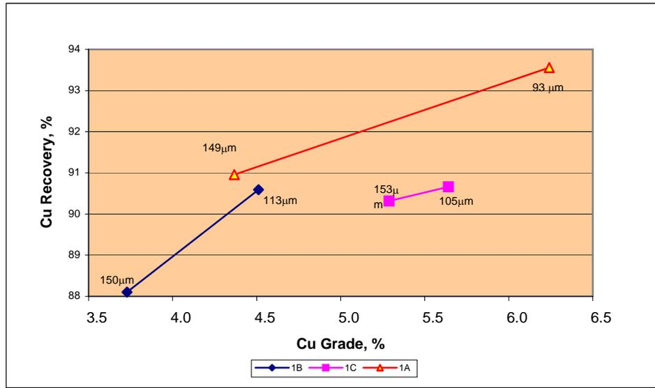
**Figure 4.2 Copper Response vs. Grind, MHM1A, B and C**
