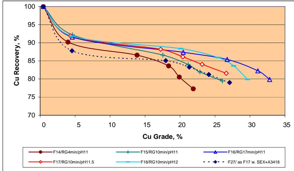
**Figure 4.14 Summary of Cleaner Tests on MHM1C**
