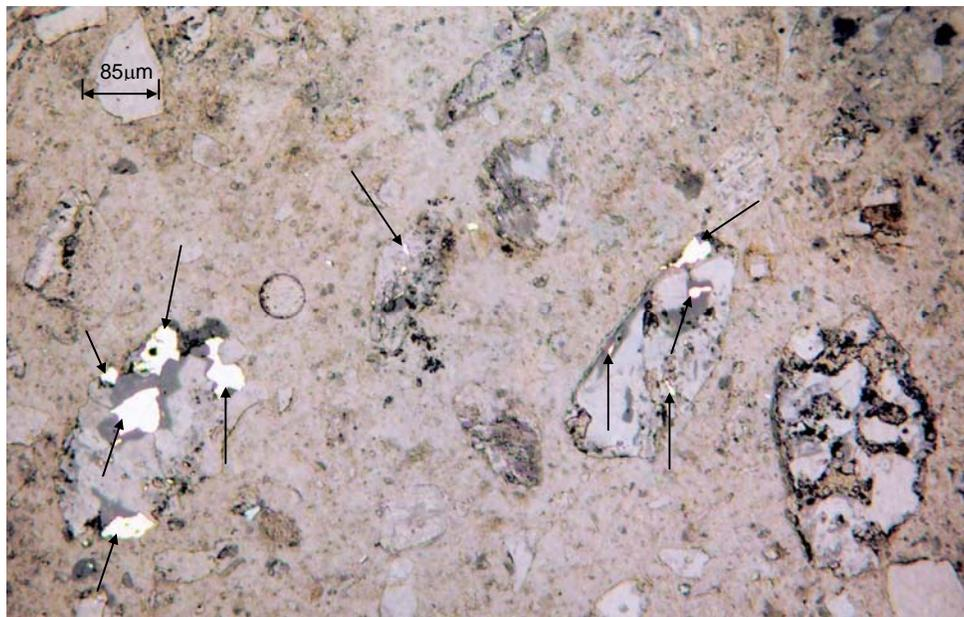
**Figure 4.10 Unliberated Chalcopyrite and Pyrite in F8 Tailings**
