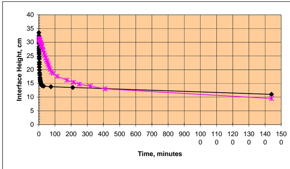
**Figure 4.18 Rougher Scavenger Tailings Settling Curves**
