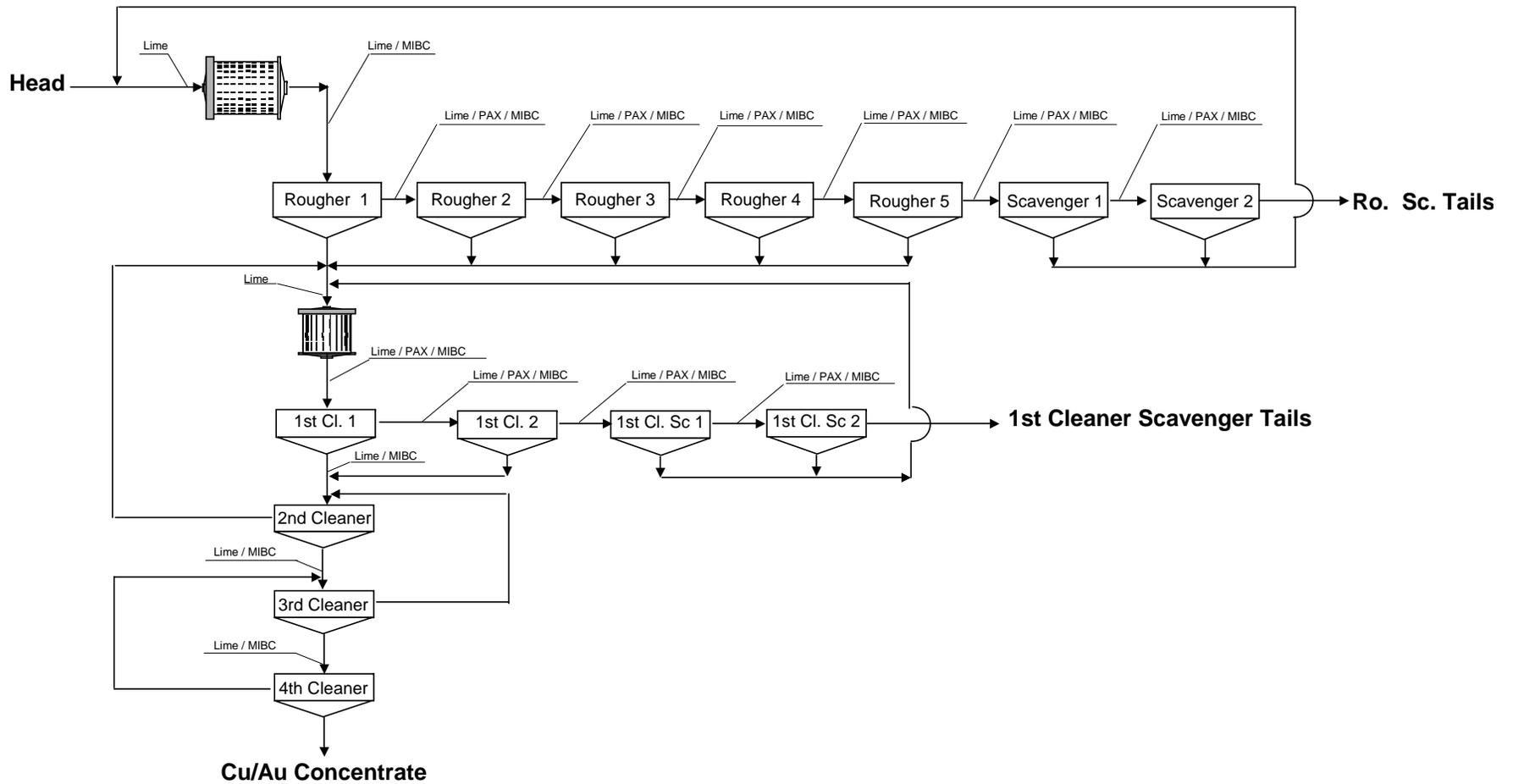
Figure 4.16 Two Tailings Rejection Flowsheet
