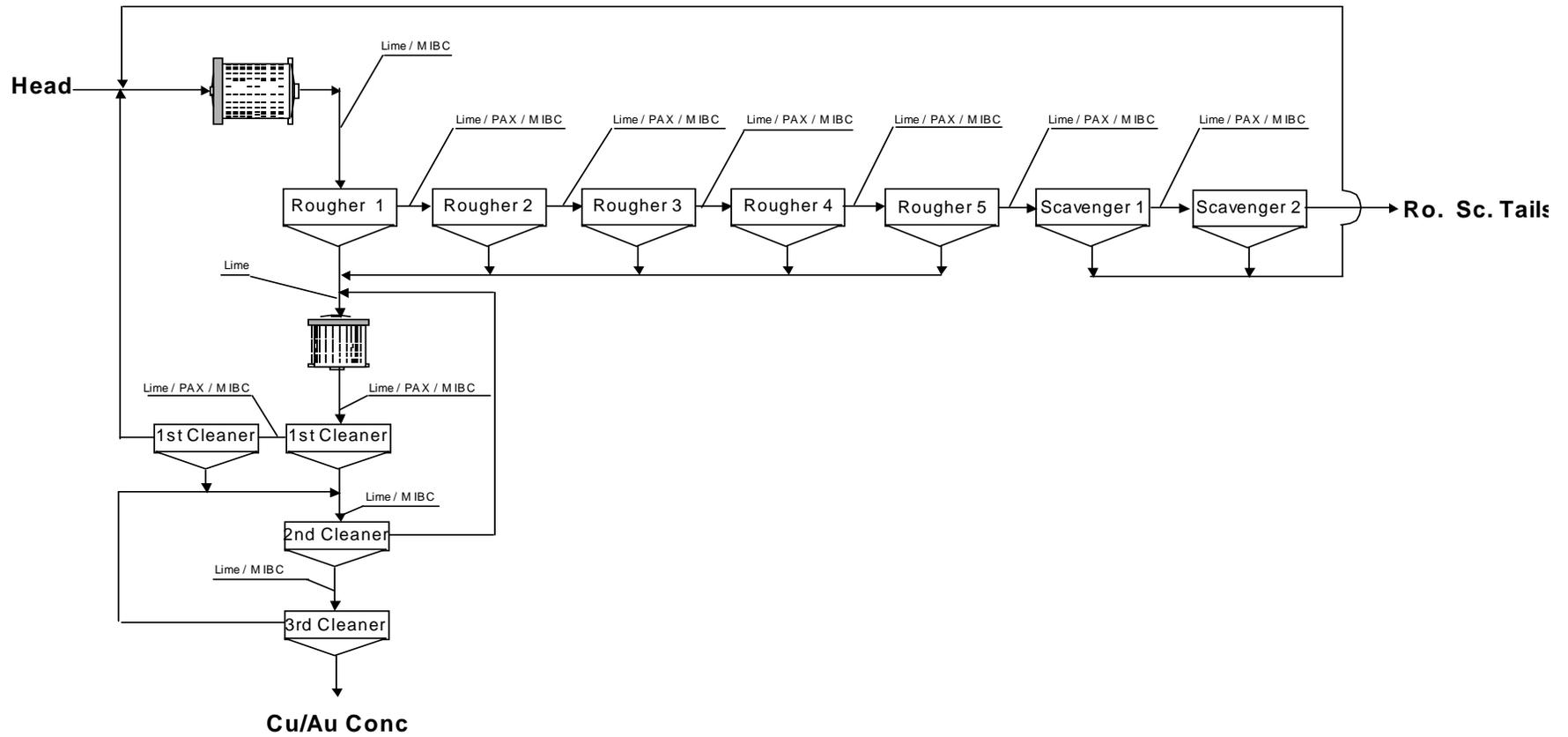
Figure 4.15 One Tailings Rejection Flowsheet
