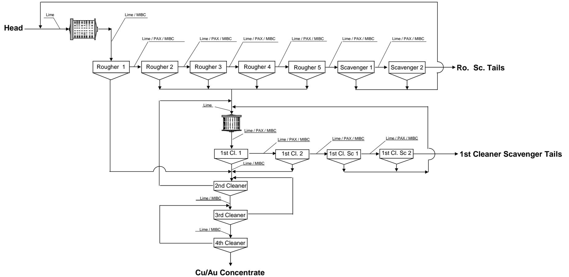
Figure 4.17 Two Tailings Flowsheet with Directing Rougher Concentrate 1 to 2<sup>nd</sup> Cleaner Flotation
