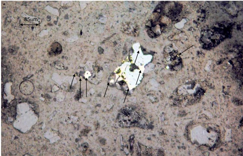
**Figure 4.9 Unliberated Chalcopyrite and Pyrite in F8 Tailings**
