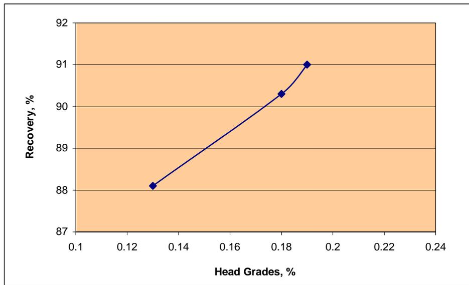
**Figure 4.3 Copper Response vs. Head Grade, MHM1A, B and C**
