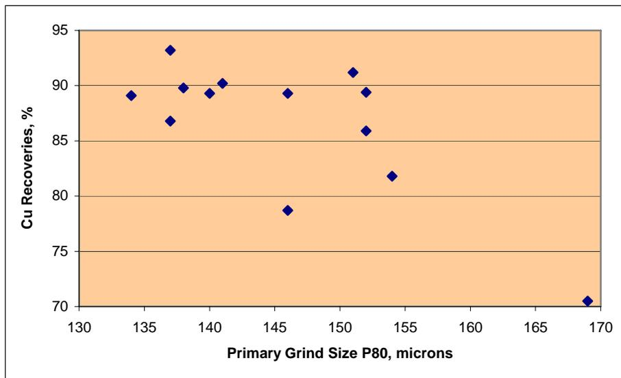
Figure 4.12 Copper Recovery vs Grind size
