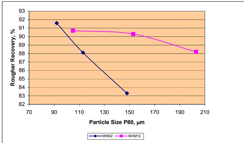
**Figure 4.4 Copper Recovery vs. Grind Size, Composites MHM2 and 1C**
