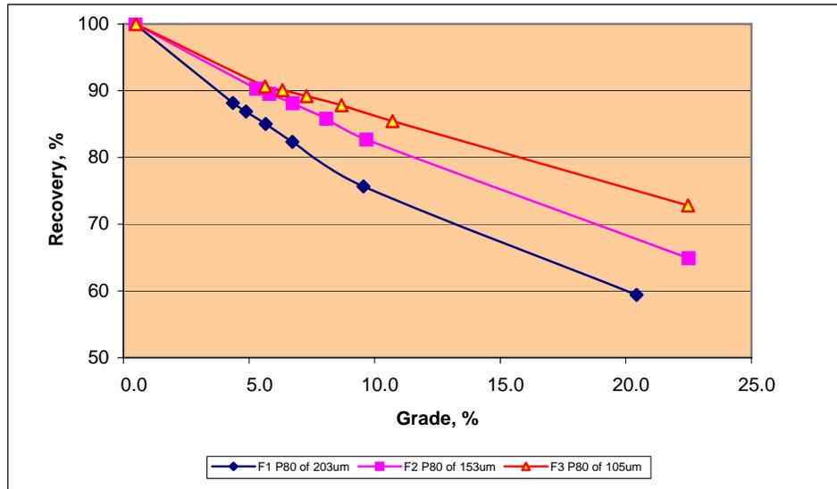
**Figure 4.1 Effect of Grind on Copper Flotation for MHM1C**
