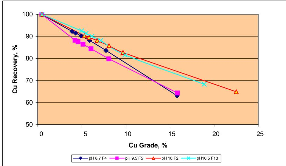
**Figure 4.6 Effect of pH on Cu Flotation for MHM1C**
